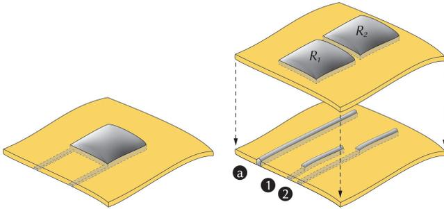
**Figure 6: Two ways provided in KnitUI for connecting knitted sensors with conductive traces:** left, for the single sensing unit, the conductive traces are knitted on the backside; right, due to the limited space, conductive traces are knitted on a separated fabric for designs with multiple sensing units. Conductive yarn is knitted on the bottom layer for the connection on the side but is only knitted around the contact area (with the sensing unit) on the top layer to avoid shorting.
