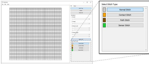
**Figure 8: Our interactive design interface:** left, the sketch where users can paint with different stitch types, where each face represents one stitch; right, the selection area that users can choose current stitch types for painting.
