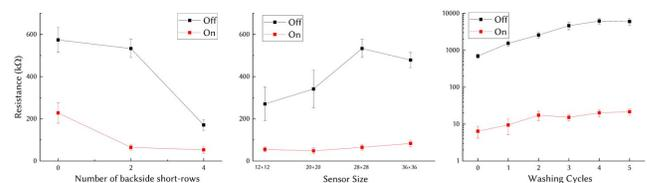
**Figure 11:** Resistance at the “ON” and “OFF” states of the sensors fabricated with different number of short-rows (left), sensing size (middle), and washing cycles (right).
