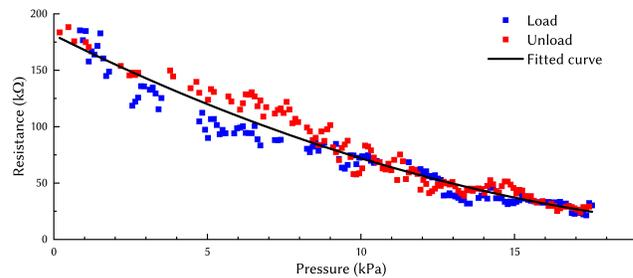
**Figure 13:** Continuous resistance profile of a typical knitted sensing unit in response to the load and unload of pressure
