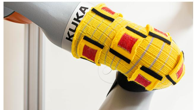
Figure 20: **Kuka with knitted sensing covering:** grey is the conductive yarn and red rectangles are sensors.
