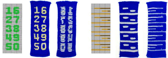
**Figure 10: An example of Numpad designed by KnitUI interface:** left, the patch with 10 separated sensors (the front and back of the corresponding knitted result), and right, the design of knitted traces to connect the sensors with the readout circuit and the corresponding fabricated result.
