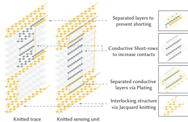
**Figure 5:** Needle  $\times$  time “bed view” for the sensing units and traces (starts from bottom). Note that we highlight each component created by knitting techniques on the right as small insets.
